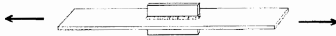
Specimen for fatigue testing: specimen contains residual stress of yield stress magnitude.
